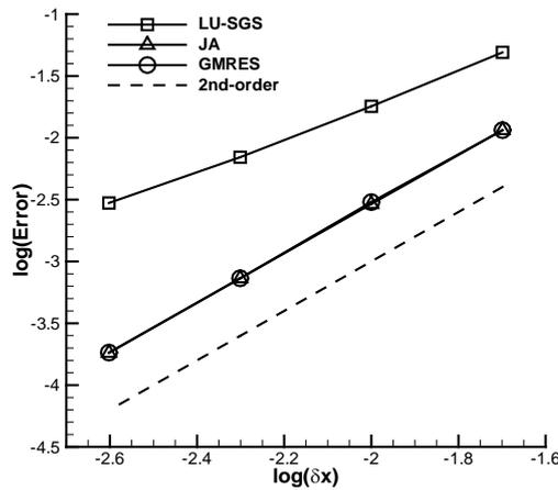
Figure 1 Errors in density vs. cell size of different time-implicit schemes.
