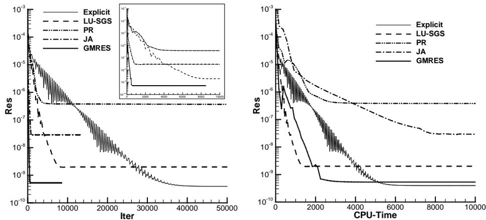
Figure 3 Computational efficiency (Left: iterations, Right: CPU-time).
