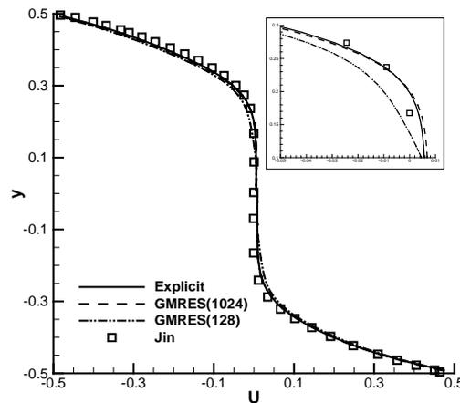
Figure 6 Velocity distributions along vertical central lines in the symmetry plane.
