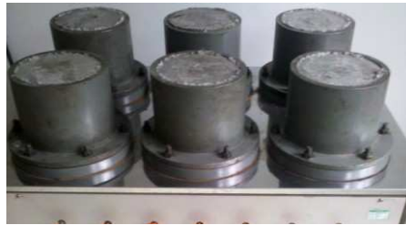
Fig 1 Concrete permeability automatic recording instrument
