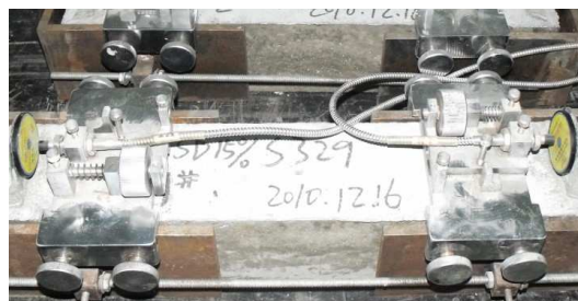
Fig 3 Non-contact concrete shrinkage test
