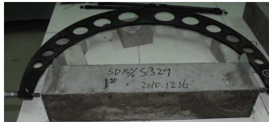
Fig 4 Contact concrete shrinkage test
