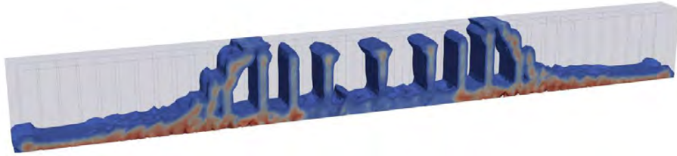
Fig.7 Failure mode obtained from simulation for the four-point test-A
