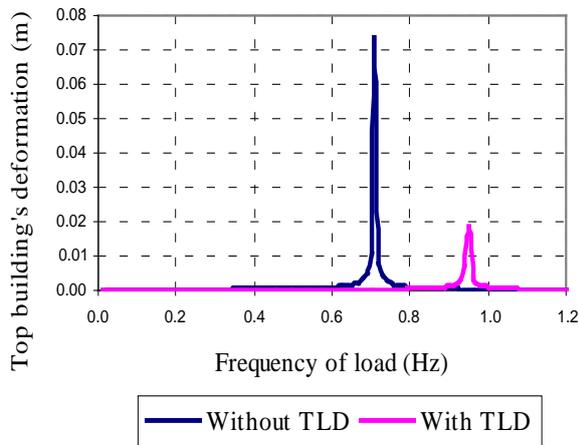
Figure 14. Structure under harmonic load
