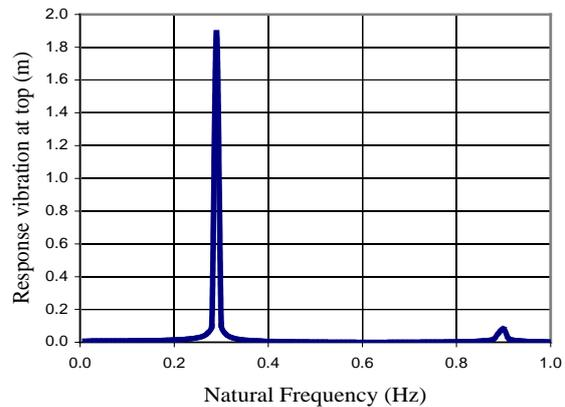
Figure 18. Response vibration of building without TLD
