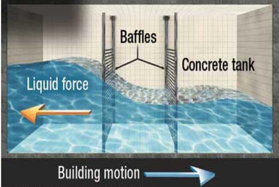
**Figure 2. Inside a liquid tank as TLD**
