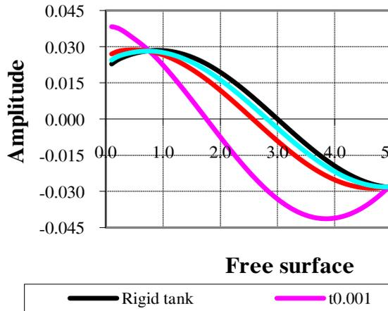
**Figure 10. Sloshing amplitude in near rigid container**
