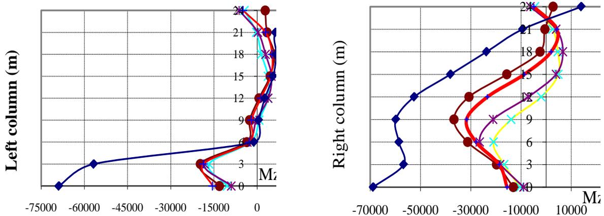
**Figure 24. Moment in left column of building**    **Figure 25. Moment in right column of building**
