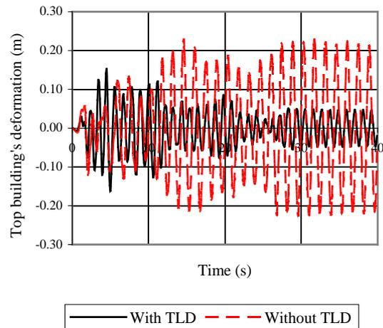
Figure 15. Structure under El-Centro
