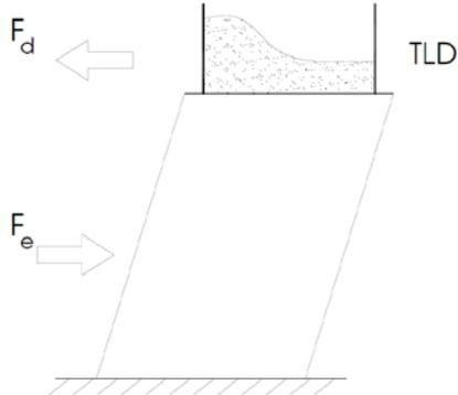
**Figure 1. Mechanism of building with TLD**
