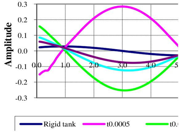
**Figure 11. Sloshing amplitude in flexible container**
