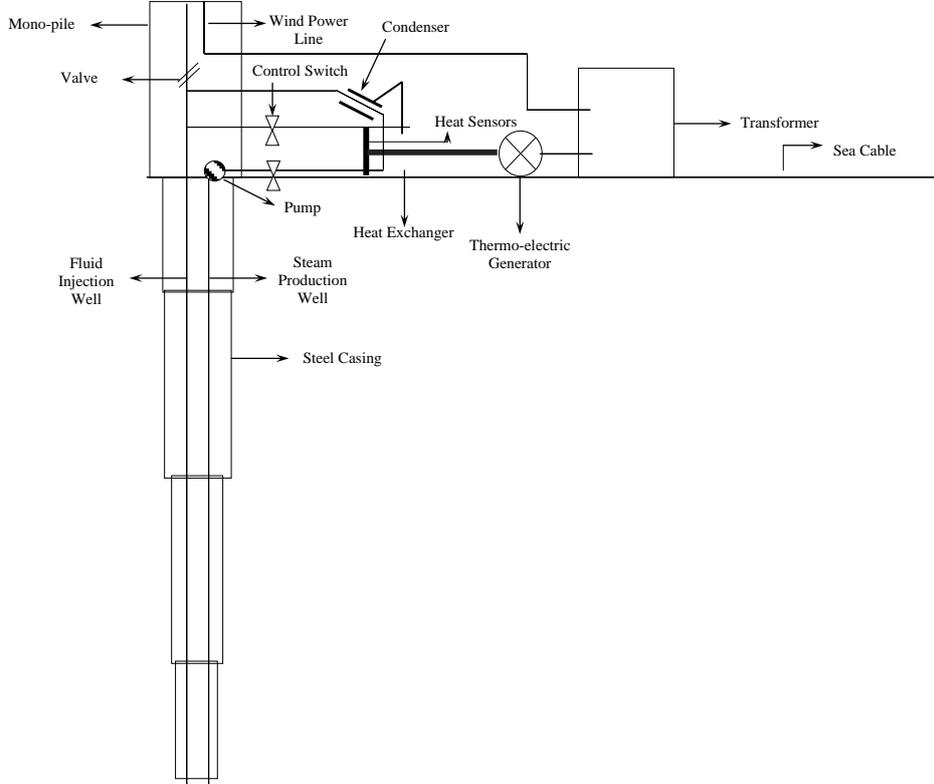
Figure 1. Schematic representation of offshore wind turbine geothermal system.
