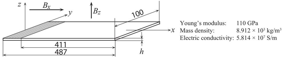
**Figure 2: Schematic diagram of a clamped plate placed in electromagnetic field.**
