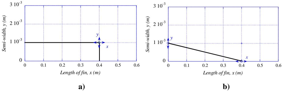
**Figure 2. The profile of fins and their optimization variables: a) rectangular fin; b) triangular fin**
