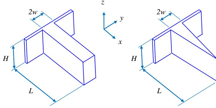
**Figure 1. The longitudinal fin with rectangular and triangular shape**
