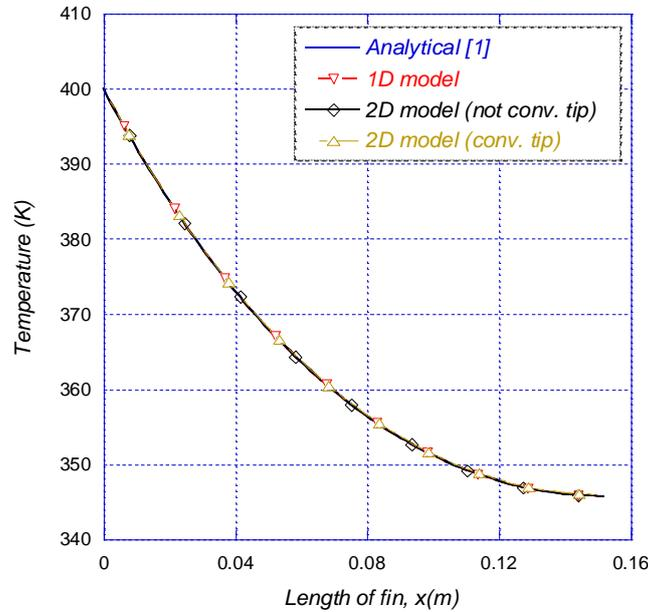
**Figure 4. The temperature distribution along the length of the optimal fin for the rectangle profile.**
