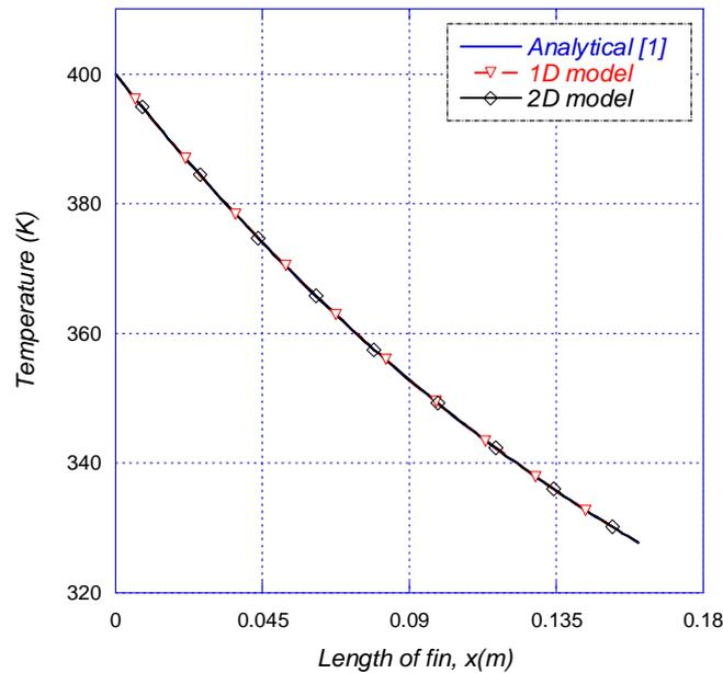
**Figure 3. The temperature distribution along the length of the optimal fin for triangle profile.**
