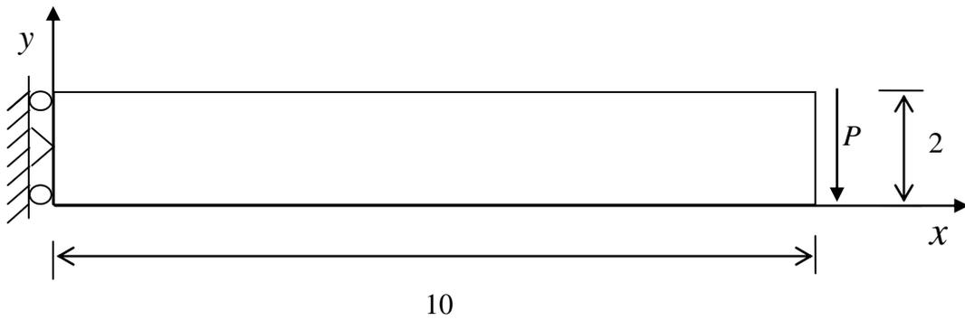
**Figure 2. Cantilever beam under a parabolic traction at the free end**
