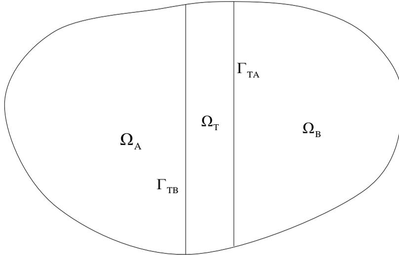
**Figure 1. The problem domain is divided into two patches and a transition region**
