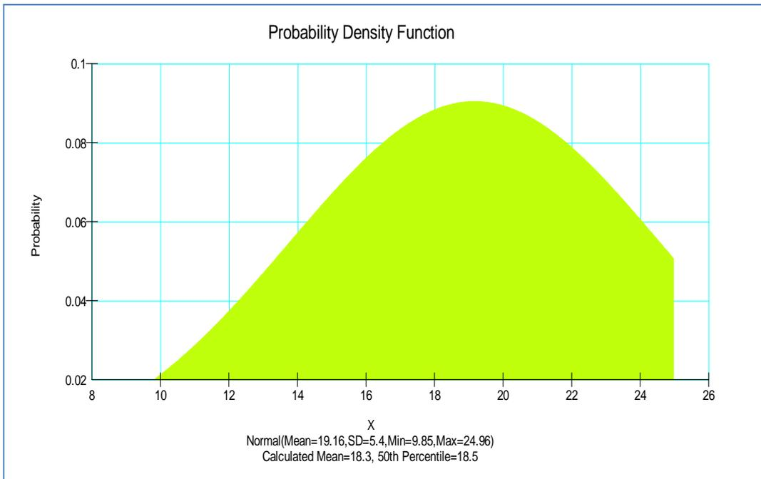
**Figure 11. Probability density function for Phi,  $\phi$  (angle of internal friction)**
