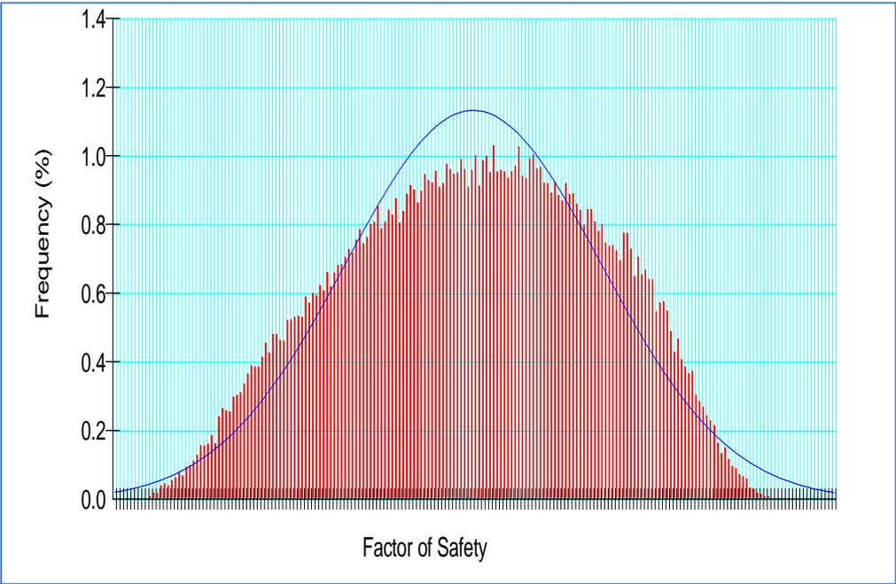
**Figure 14. Probability distribution for factor of safety at section 3-3**
