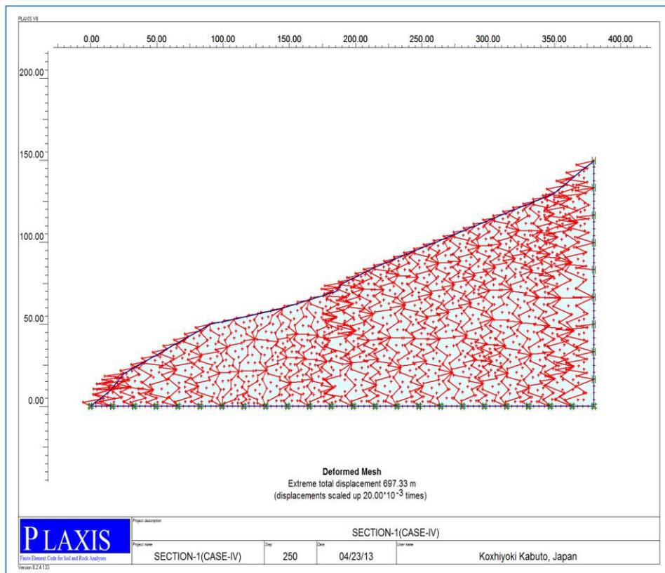
**Figure 6. Deformed mesh at section 1-1 with dynamic loading at most critical plane**
