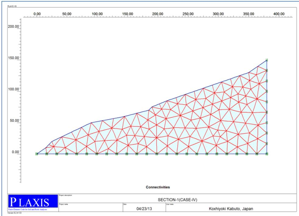
**Figure 5. Finite element modeling at section 1-1 with dynamic loading at most critical plane**
