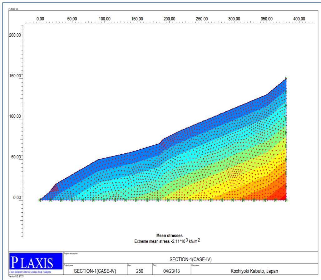
**Figure 7. Stress distribution at section 1 with dynamic loading at most critical plane**
