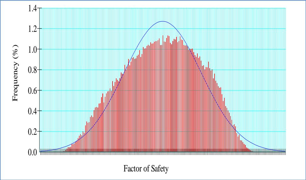
**Figure 13. Probability distribution for factor of safety at section 2-2**
