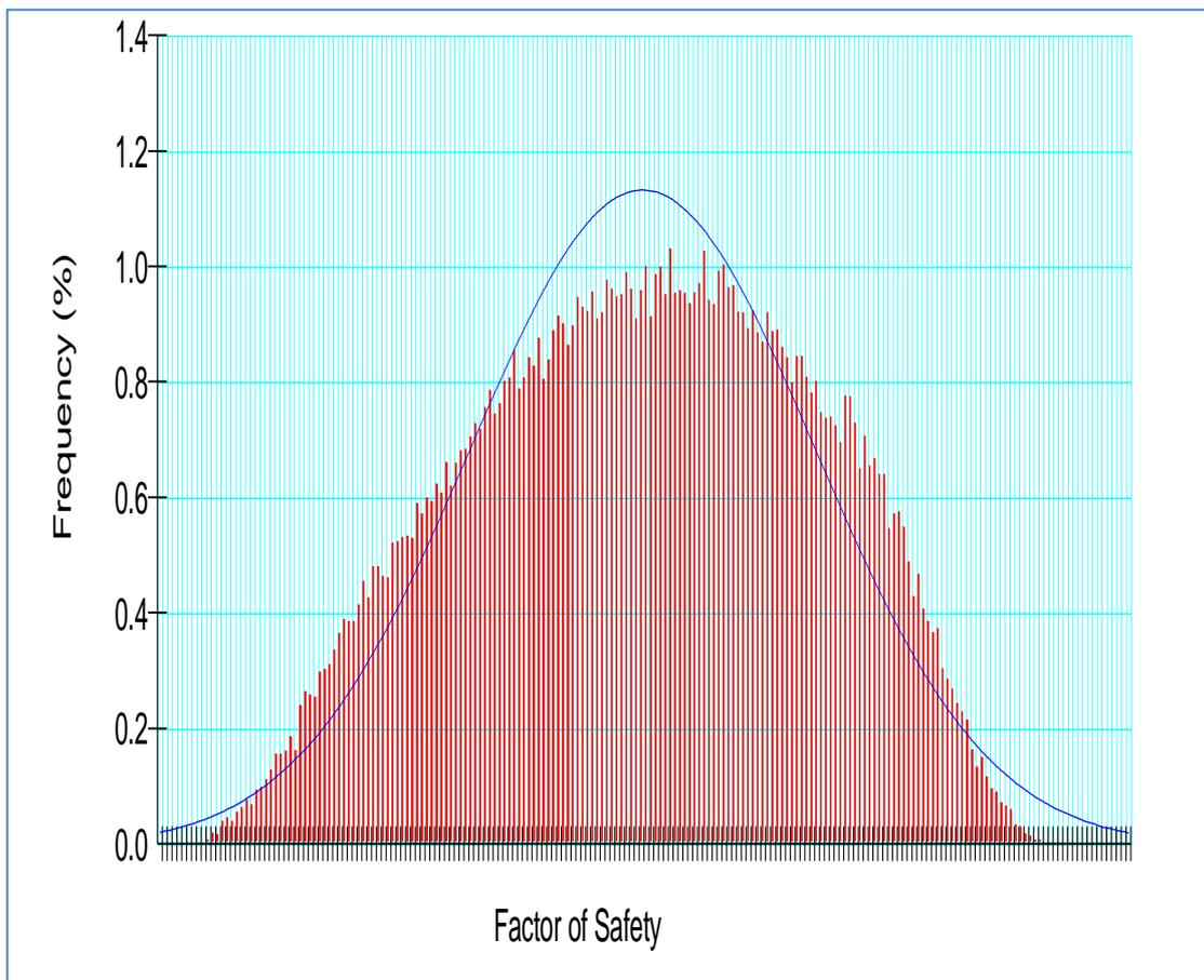
**Figure 12. Probability distribution for factor of safety at section 1-1**
