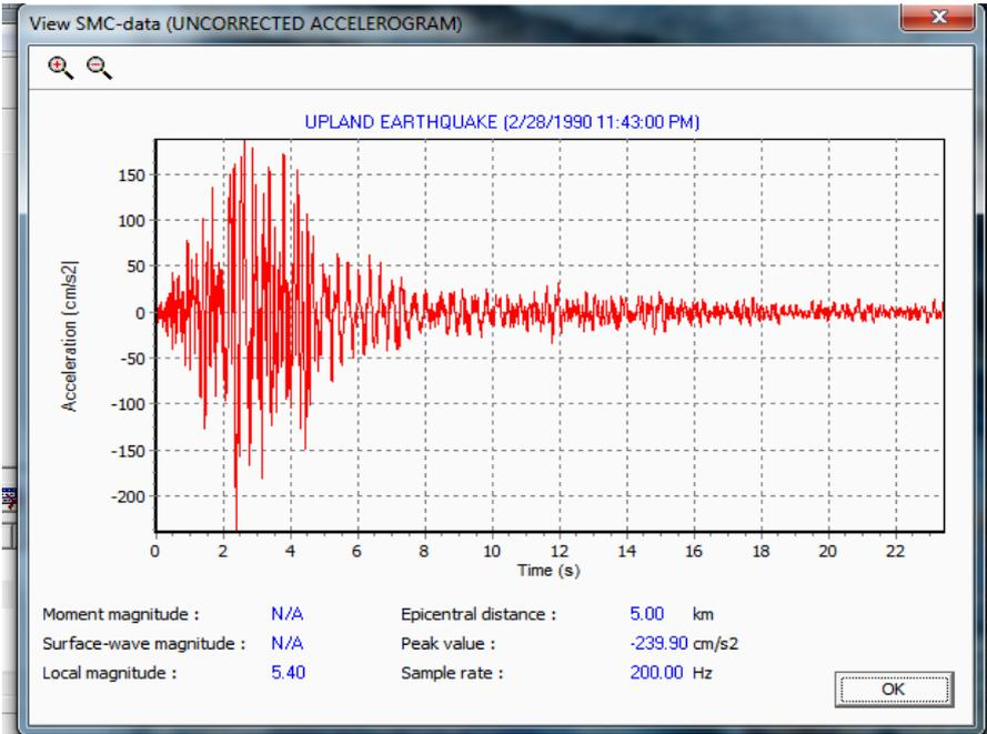
**Figure 4. Accelerogram used to simulate dynamic loading input**
