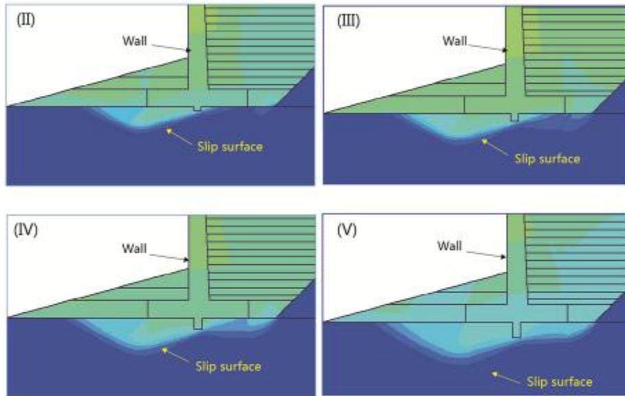
**Figure 7 Total displacement contours for CRWs with different shear key lengths**
