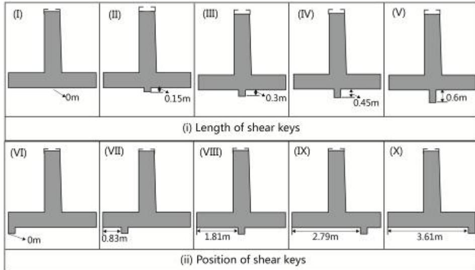
**Figure 5. Ten types of shear keys considered in this paper**
