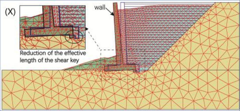
**Figure 10 Grid deformation of the CRW with a shear key at the end of the heel**
