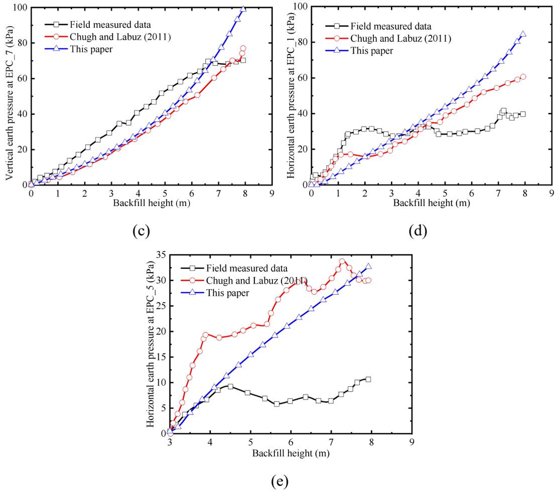
**Fig. 4 Comparison between the results in this paper, the field measured data and the results from the literature [2]: (a) Horizontal displacement of the CRW; (b) Vertical earth pressure of EPC\_9; (c) Vertical earth pressure of EPC\_7; (d) Horizontal earth pressure of EPC\_1; (e) Horizontal earth pressure of EPC\_5.**
