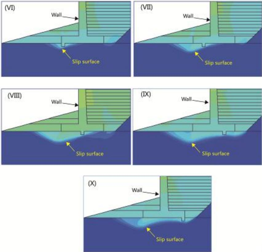
**Figure 9 Total displacement contours for CRWs with different shear key positions**
