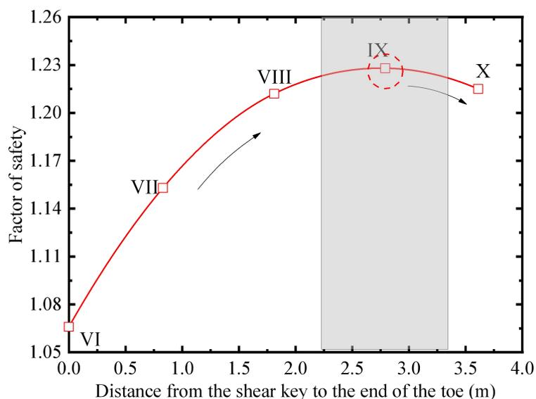
**Figure 8 Variation curve of the factor of safety of the CRWs with different shear key positions**
