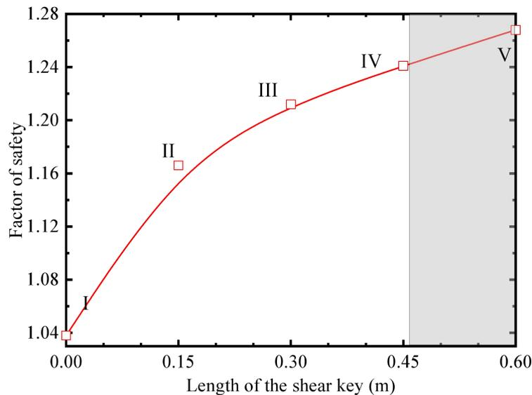
**Figure 6 Variation curve of the factor of safety of the CRWs with different shear key lengths**
