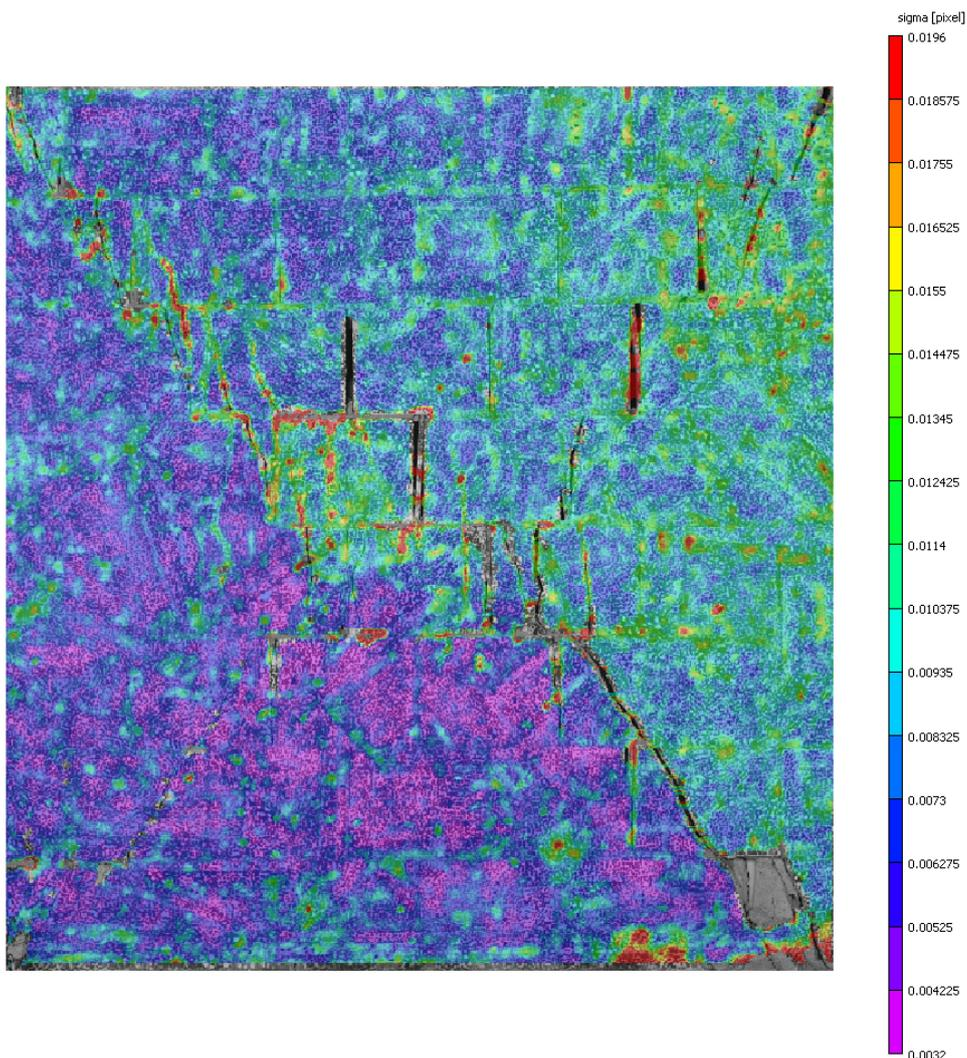
**Figure 5. Confidence interval, in pixels, in wall P4**
