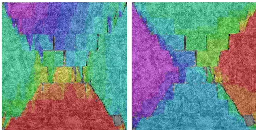
**Figure 3. Vertical (left) and longitudinal (right) displacement fields in wall P4**
