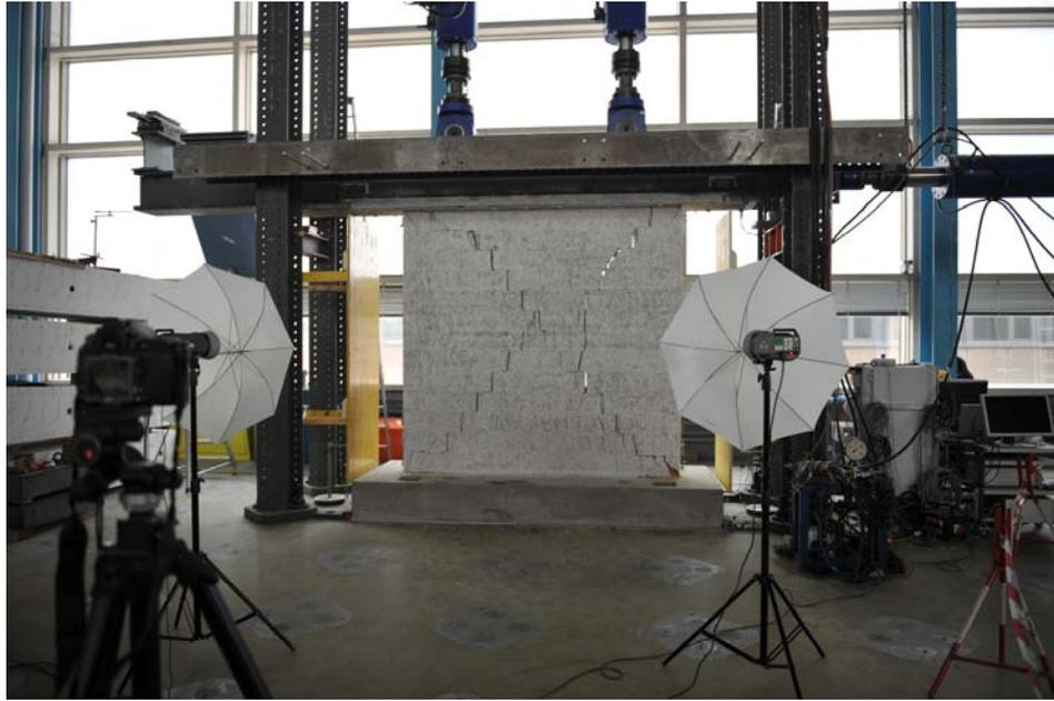
**Figure 1. Test set-up with tested wall T2**
