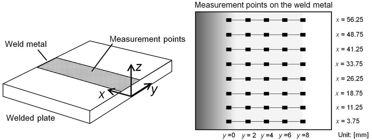
**Figure 6. Measurement points on the weld metal**
