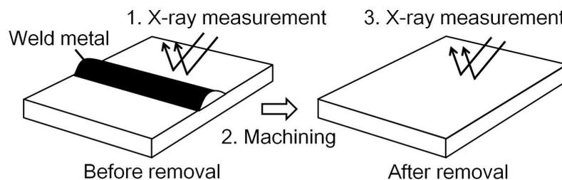
**Figure 1. Procedures in the advanced bead flush method**
