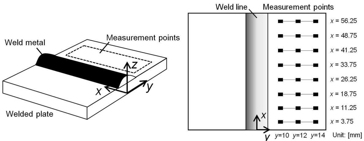
**Figure 5. Measurement points on the base metal**
