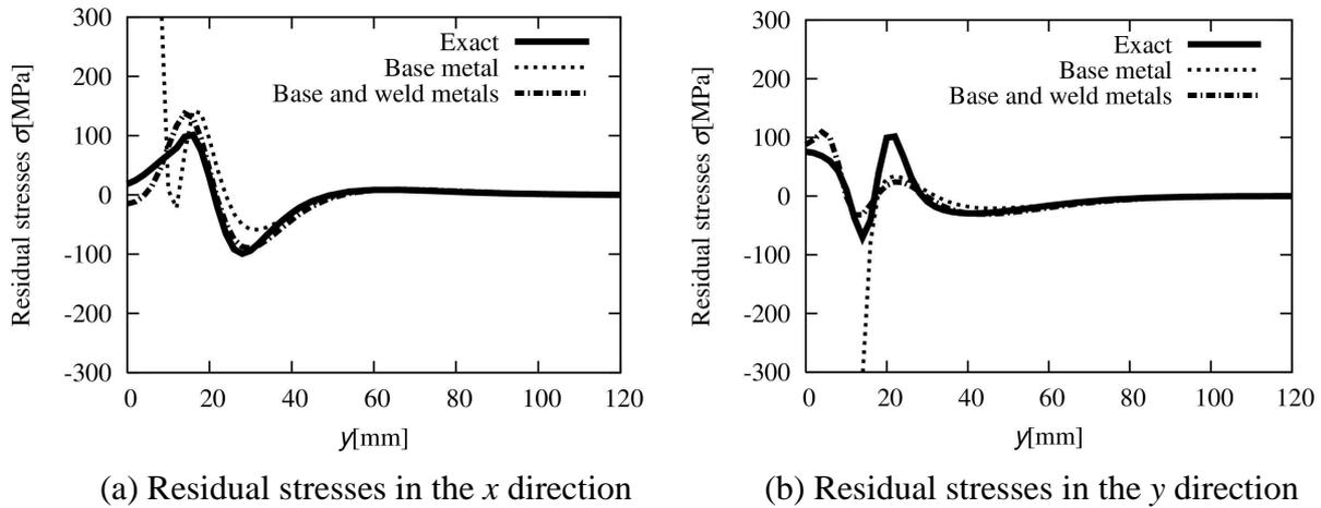
**Figure 7. Estimated residual stresses on the bottom surface after the removal. The dotted and chain lines are estimated results from residual strains on the base metal and on the base and weld metals, respectively.**
